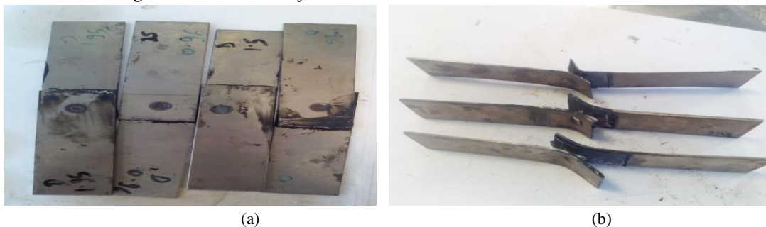
Fig.8: The weld bonded joints before tensile-shear test (a) and (b) after tensile shear test
